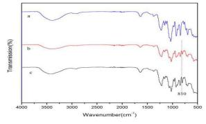
Figure 1. FTIR spectrum of carrageenan((a). Commercial κcarrageenan;(b). Carrageenan extracted from *Chondrus*; (c). Commercial ι-carrageenan)
