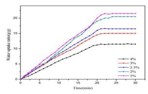
Figure 3. Relationship between water absorption ratio and absorption time of carrageenan aerogels with different carrageenan concentrations
