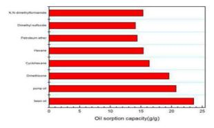
Figure 4. Organic solvents absorption capacity of carrageenan aerogel with 2.5wt% carrageenan concentration
