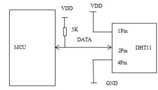
Figure 2 Typical interface connection diagram
