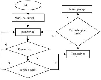
Figure 7 Terminal Workflow Diagram
